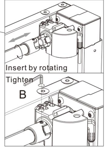
Connect transmission rod(7) with column (1)&(2), first according to way 1, then way 2, meanwhile use 2.5x2.5 wrench (B) to tighten.
