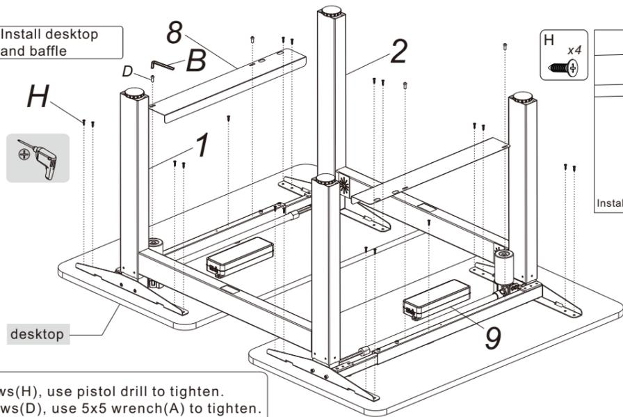
Connect desktop by screws(H), use pistol drill to tighten. Connect baffle(8) by screws(D), use 5x5 wrench(A) to tighten.
