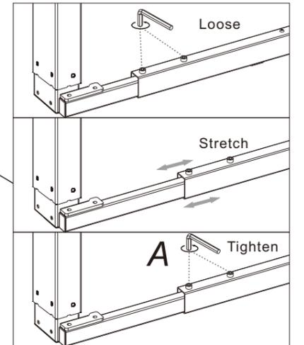
Install supporting beam(5), use 5\*5 wrench(A) to tighten the screws(F).
