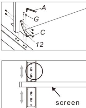
Adjust place of screen fixing base (12) according to the thickness of screen, use 5x5 wrench(A) to tighten the screws(G).
