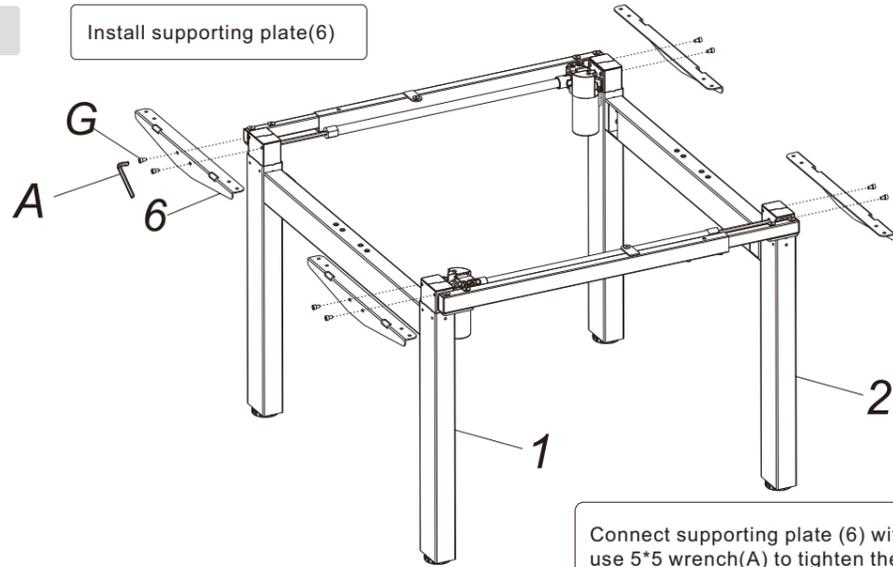
Connect supporting plate (6) with column(1)&(2), use 5\*5 wrench(A) to tighten the screws(G).
