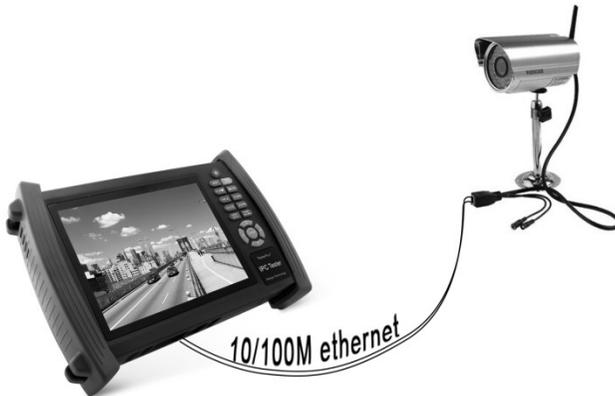
Note: if IP camera not support external power supply, but only support PoE power, then connect to tester LAN port to supply PoE Power for IP camera. Before connecting, the network switch and tester must be disconnecting status. It means PSE port cannot be connected to any network cable if supply PoE power
