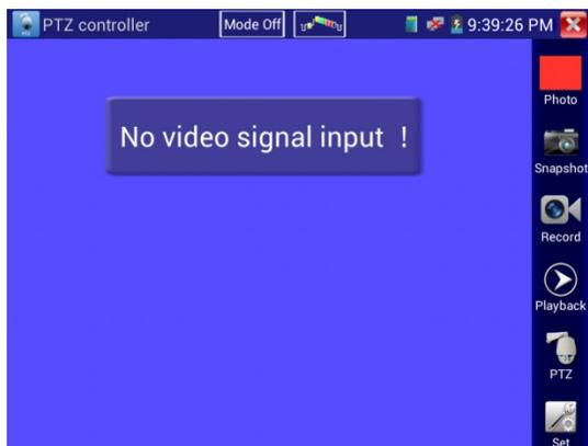
Display the input video images, Select relative function in the right side Toolbar to operate , with ”camera ”,“Recording”、 “Photos”、 “Video playback”,”PTZ control”、 “color and storage setting ” function .
