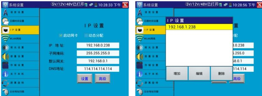
After setting IP address (ref above pictures), it can test two network segments IP camera (192.168.0.0and) 192.168.1.0.
