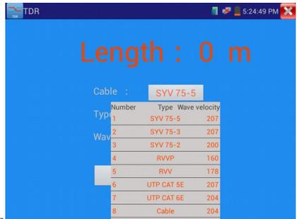
User-defined calibration: Choose the cable 100 meters to 200 meters (more than 50 meters) ,click cable type to select user-defined 1 for calibration, 11 groups user-defined can be set.
