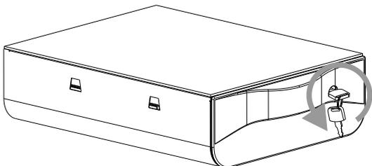
Close the drawer and then rotate the key 90 degree counterclockwise to lock the drawer.
