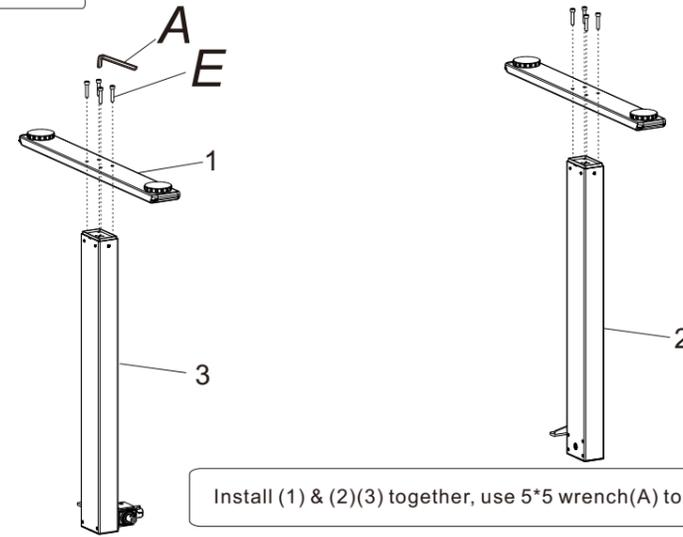
Install (1) & (2)(3) together, use 5\*5 wrench(A) to tighten the screws(E).
