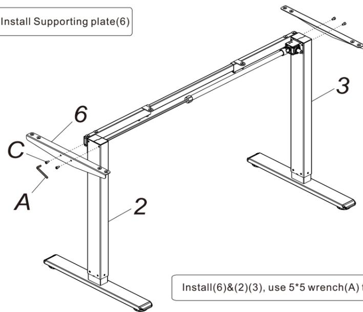
Install(6)&amp;(2)(3), use 5\*5 wrench(A) to tighten the screws(C).
