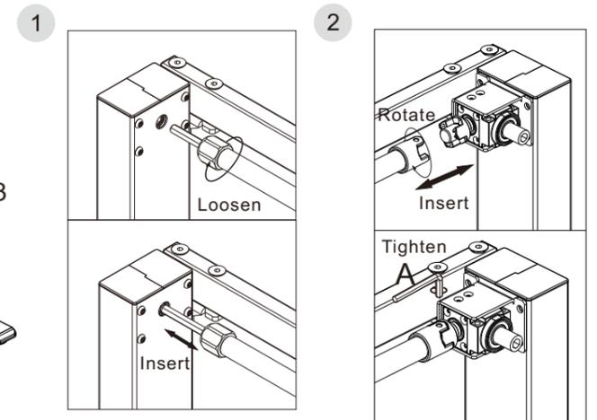
Do not rotate the drive rod more than a third of a turn.
