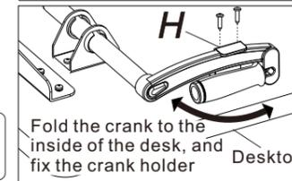
Fold the crank to the inside of the desk, and fix the crank holder (H) on the Desktop
