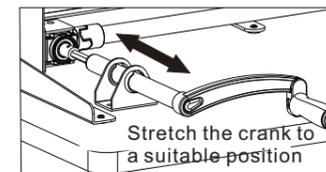
Stretch the crank to a suitable position
