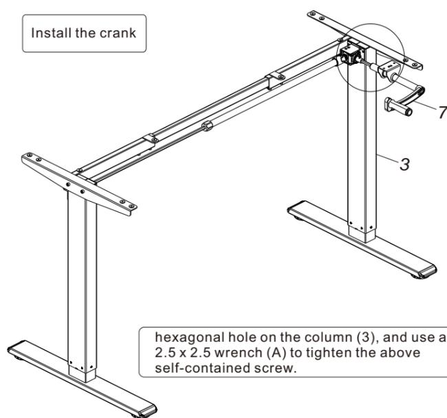
hexagonal hole on the column (3), and use a 2.5 x 2.5 wrench (A) to tighten the above self-contained screw.
