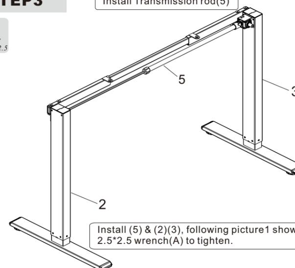
Install (5) & (2)(3), following picture 1 shows first, then picture 2, use 2.5\*2.5 wrench(A) to tighten.
