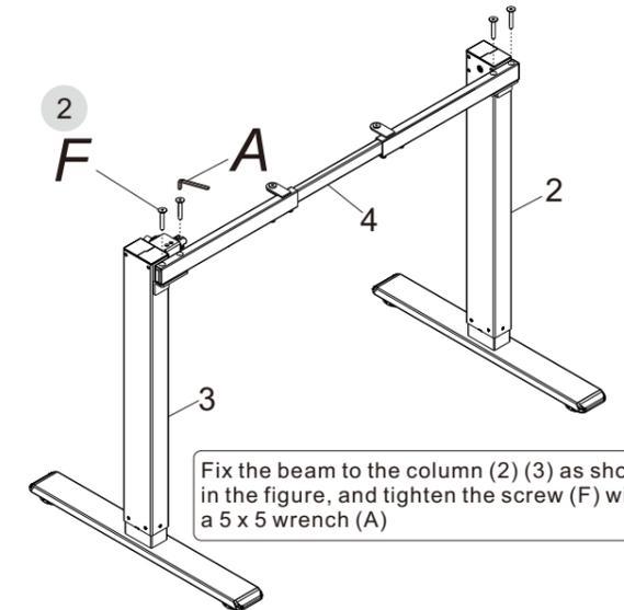
Fix the beam to the column (2) (3) as shown in the figure, and tighten the screw (F) with a 5 x 5 wrench (A)
