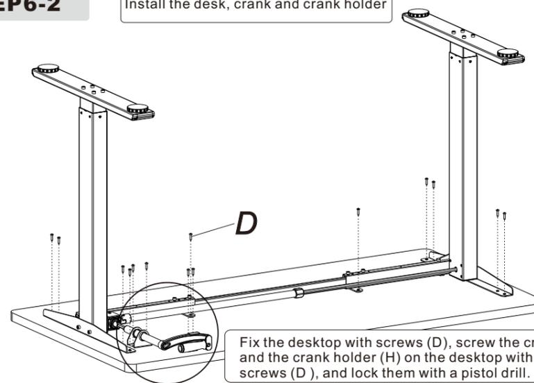
Fix the desktop with screws (D), screw the crank (7) and the crank holder (H) on the desktop with screws (D), and lock them with a pistol drill.
