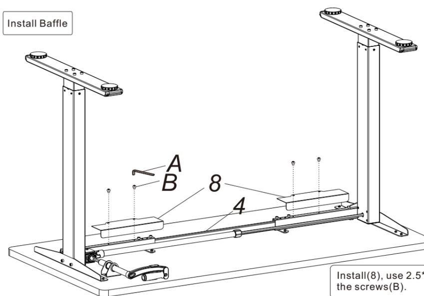
Install(8), use 2.5\*2.5 wrench(A) to tighten the screws(B).
