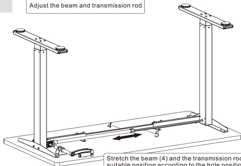
Stretch the beam (4) and the transmission rod (5) to a suitable position according to the hole position of the desk.
