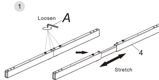
Loosen the 4 screws on the beam (4) with a 4 x 4 wrench (A), and then pull the beam apart
