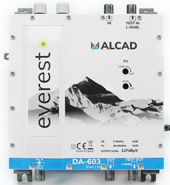
Broadband distribution amplifier for terrestrial TV (117 dBuV). It has a gain control and variable slope control. It amplifies the return path from 5 to 65 MHz. Fed by an external power supply model FF-200 (included with the amplifier). The input and output test points permit checking and adjusting the installation with no need to disconnect the TV signal.
