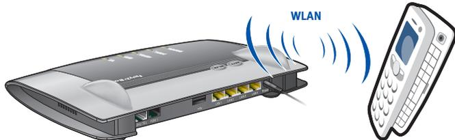
Connecting an IP telephone with the FRITZ!Box over WLAN
