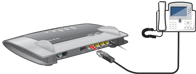
Connecting an IP telephone to the network port of the FRITZ!Box
