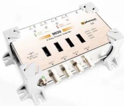
The 9930 is a **satellite power inserter**, which can be used to ensure a universal LNB is locked on the correct satellite band. Each of the 4 inputs can be configured to deliver the desired control signals (13/18V + 0/22 kHz). The selected control signal is indicated by a bi-color LED.
