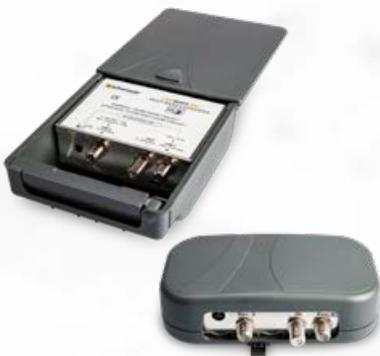
The **Stacker-Destacker** is the perfect solution to upgrade an old single-cable system with a twin (or quad) LNB to be used in combination with a dual input receiver (PVR) or 2 separate single input receivers. The advantage of using the Stacker-Destacker is that you don't need an additional cable. The Stacker converts the frequencies of the second input, so it is literally stacked above the frequencies of the first input. The Destacker converts the frequencies back to the original ones.
