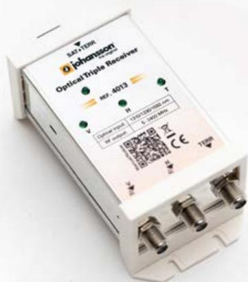
The **optical receiver** is developed for the transmission of wideband signals in medium and large Fiber Optic systems. The Optical receiver can convert one, two or three wavelengths. Ref. 4011 (Optical Single Receiver) converts 1550nm to Satellite or Terrestrial signal. Ref. 4012 (Optical Dual Receiver) converts 1310 + 1330 nm to wideband V/H; Ref. 4013 (Optical Triple Receiver) converts 1310 + 1330 + 1550 nm to wideband V/H and Terrestrial signal.
