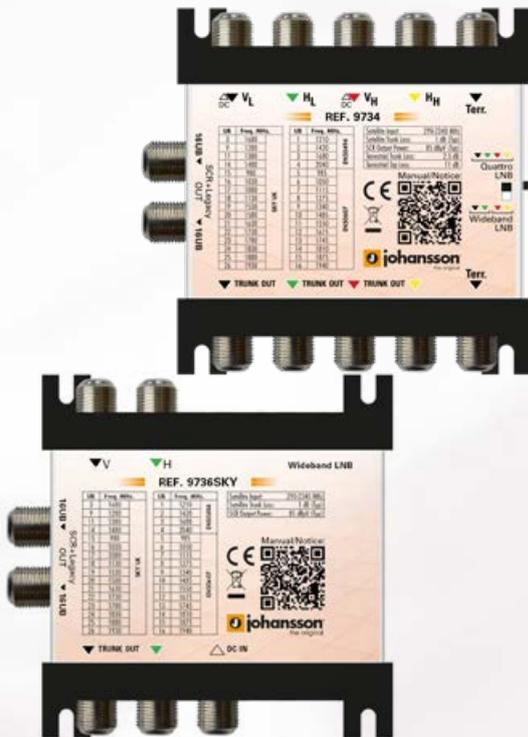
The 9734 has 4 satellite wideband input (for 1 quattro or 2 wideband LNB), passive terrestrial diplexer, 2 outputs with each 16 user bands.
